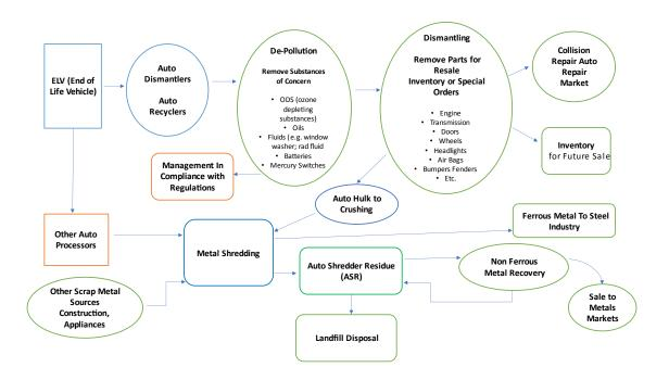
Figure 1: Auto Recycling Schematic
