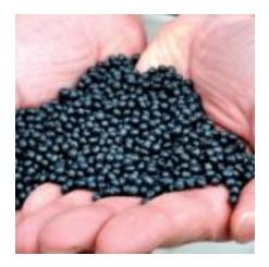
Figure 1: Plastic Output from Ad Rem ASR Sorting Technology<sup>72</sup>
